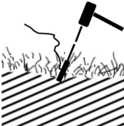
4. Slide the swage onto the cable (be careful not to let the swage/crimp slide into the hole in the ground).
